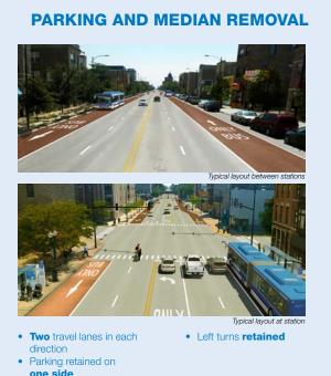
This BRT Alternative includes one curbside running bus lane in each direction, two automobile travel lanes in each direction, and parking on one side. One side of parking is removed as well as all medians. Sidewalk widths remain the same and curb extensions are provided at station intersections. Existing medians will be retained or reconstructed. All left turn lane pockets and approximately 25 percent of left turn lanes will be retained.
