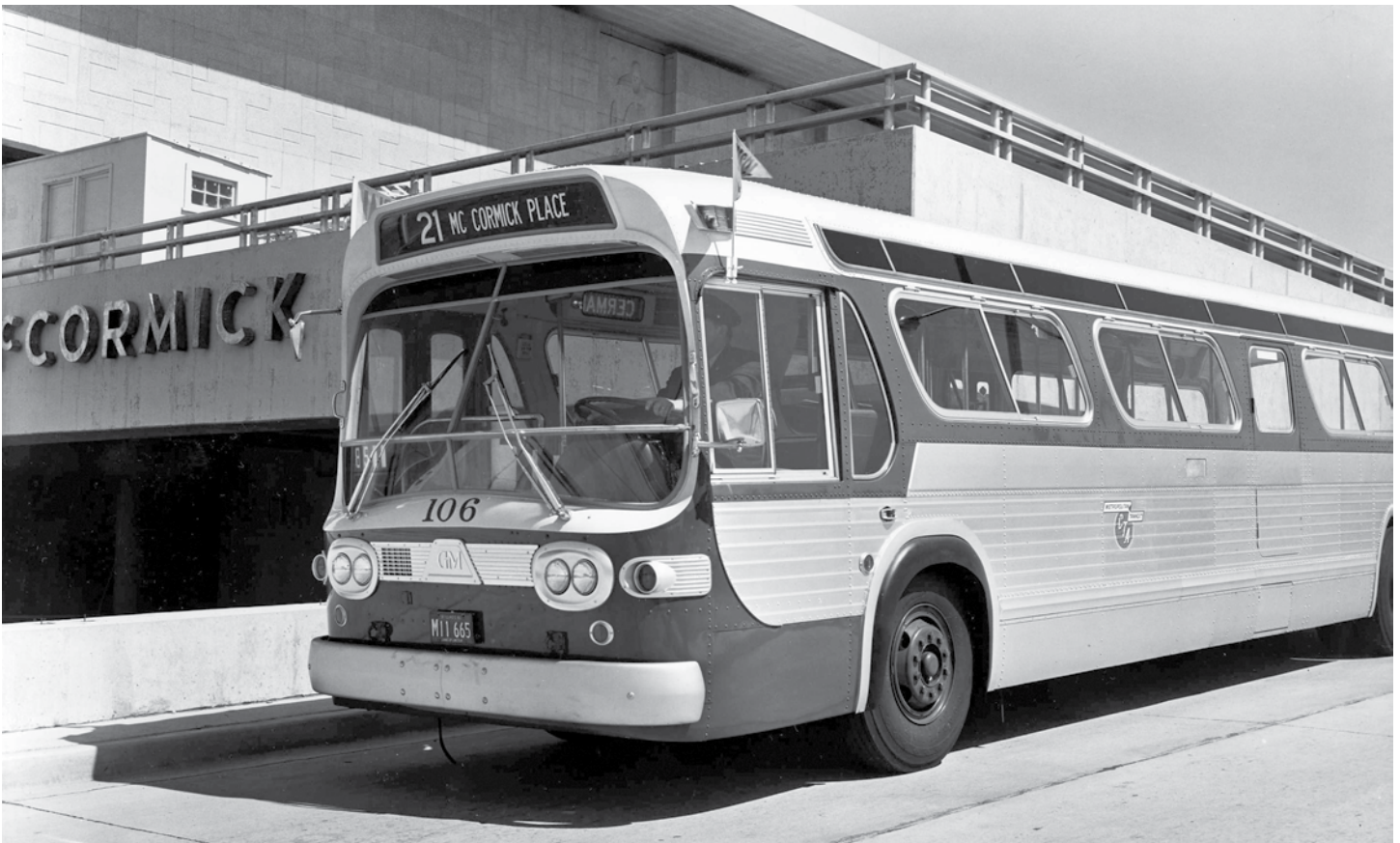
CTA #106 is pictured next to the original McCormick Place, which opened in November 1960. Manufactured by General Motors in 1961, this “New Look” bus included a number of progressive features such as large, double windows, fluorescent lighting and bright interiors. The bus is working the “Green Pennant Special,” a special event route that operated between McCormick Place and the Loop during the 1960s. At the time, there was no direct bus service from the Loop to McCormick Place, so for some conventions and trade shows this special express route was operated via Lake Shore Drive. The buses were marked with green pennants on the front that said “SPECIAL”.
