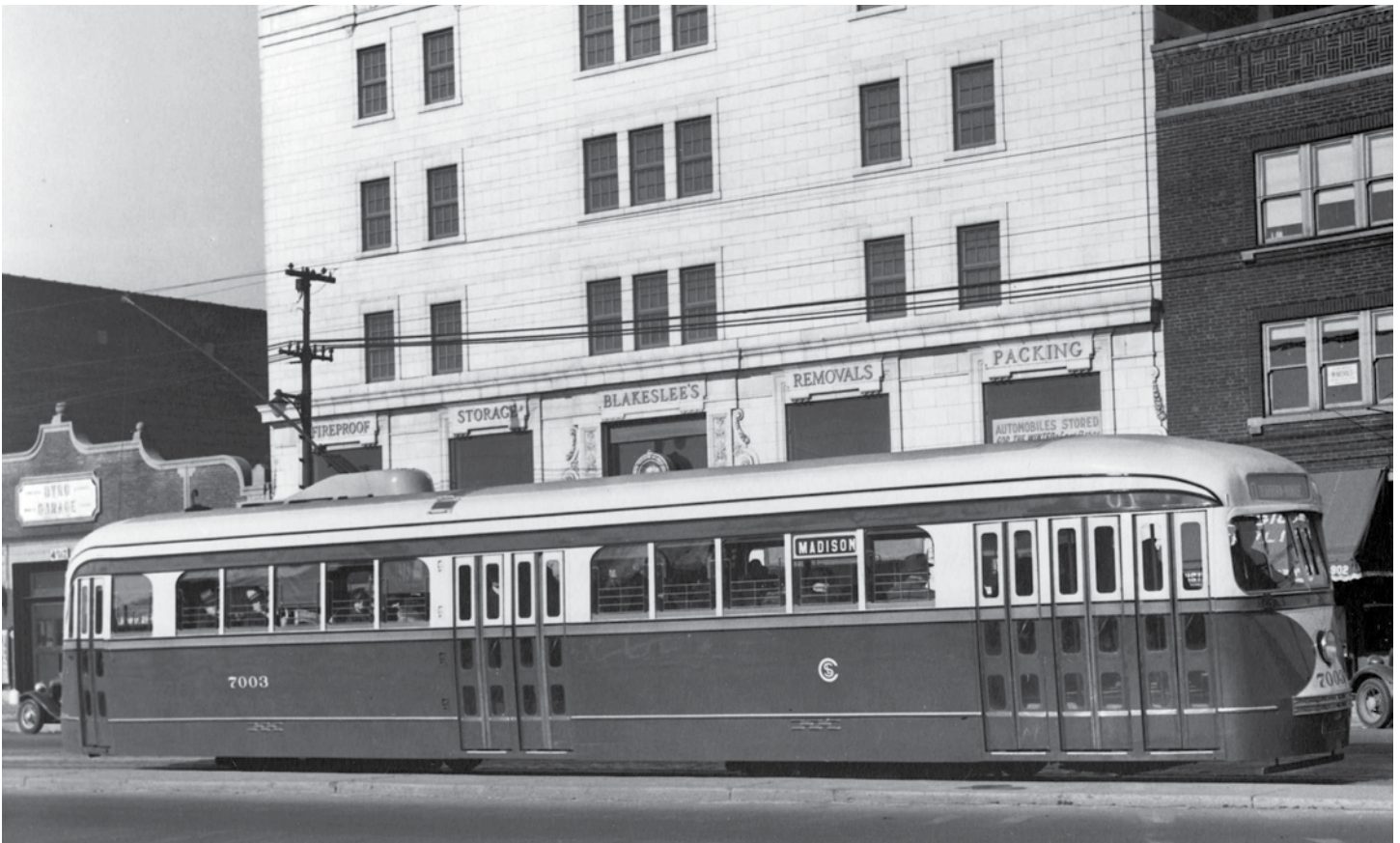
Chicago Surface Lines "Blue Goose" streetcar #7003, one of 83 built in 1936 by the St. Louis Car Company, heads toward the Loop along Madison near Cicero. The #20 Madison route was the first to receive these cars, nicknamed PCC cars for the Presidents Conference Committee. The Committee, comprised of the heads of the various street railways in North America, developed a standardized state-of-the-art streetcar design to provide a modern vehicle that would appeal to the public and be economical to produce. PCCs saw service in many American cities, including Chicago, Brooklyn, Baltimore, Boston and Pittsburgh.
