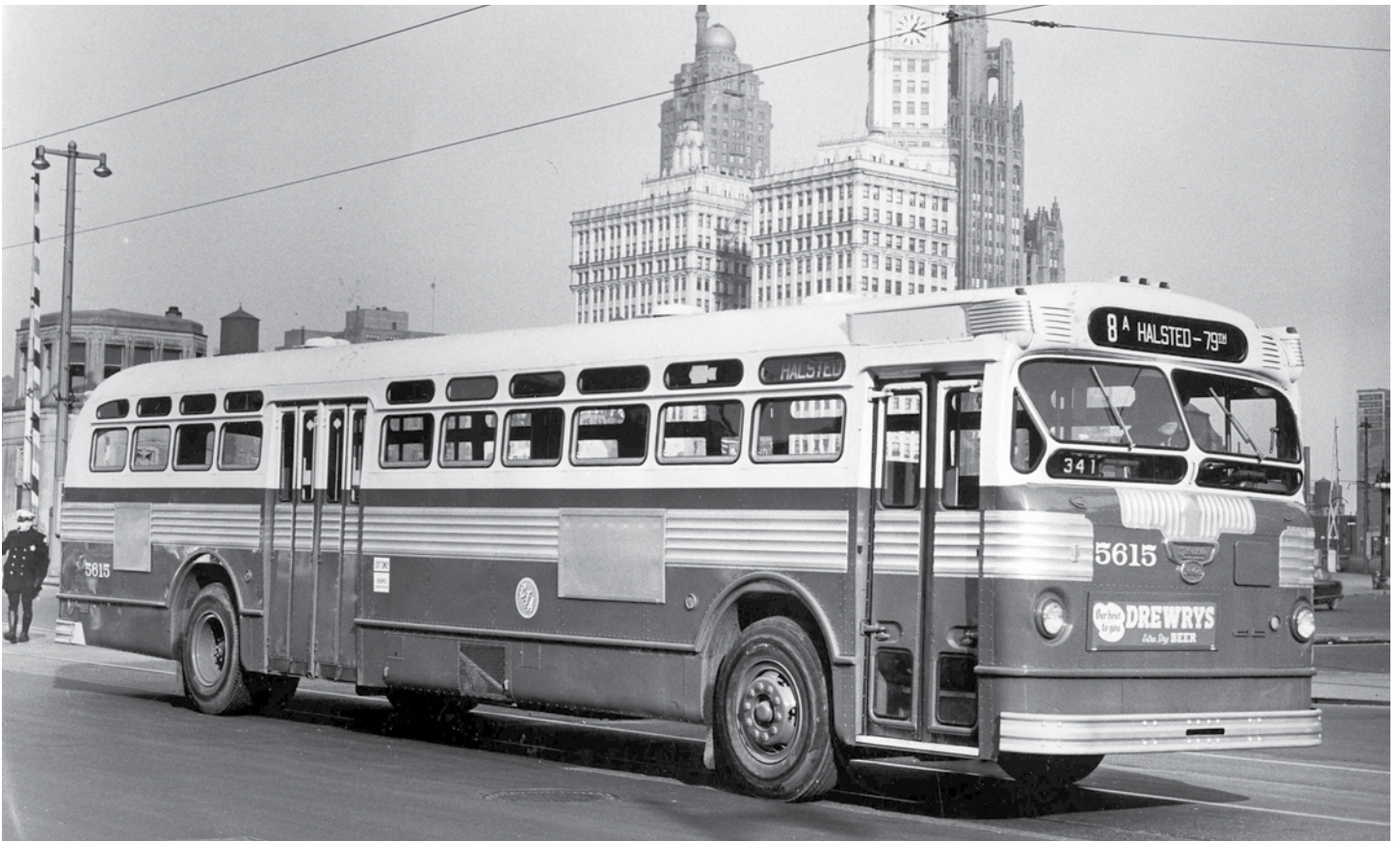
CTA Flxible Twin Coach bus #5615, manufactured by the Flxible Company in 1953, is posed on State Street at Wacker Drive. These buses were fueled by liquefied petroleum gas (propane). Chicago was one of the largest users of propane buses, with a fleet of 1,700, built by such companies as Fageol Twin Coach, Flxible, Mack, and ACF-Brill between 1950 and 1962. No doubt photographed to promote the modernization of CTA's fleet, the staged nature of the photo is revealed by the bus's destination signs – route #8A is a south extension of the Halsted Street bus and begins about 10 miles south of State and Wacker! The route designation #8A also didn't come into use until more than 20 years after the photo was taken; the route was designated #42B at the time.
