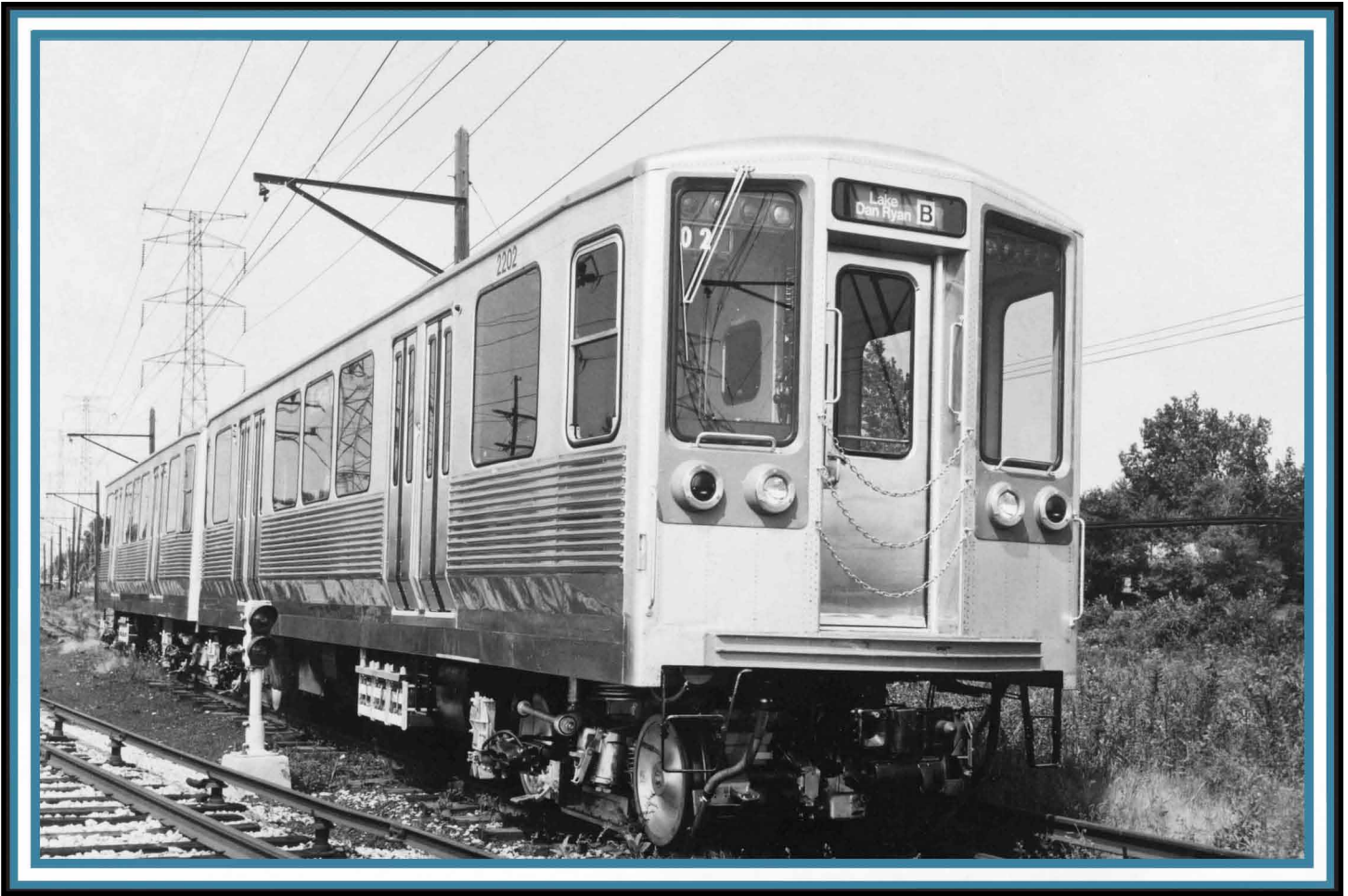
In this photo, rapid transit cars 2201-2202 are seen on the Skokie Shops freight lead, newly arrived from the Budd Company, the first two cars of an order of 150 cars delivered in 1969 and 1970. The delivery of these cars coincided with the opening of the new Dan Ryan line and the extension of the Milwaukee route to Jefferson Park in 1969 and 1970, respectively. With their rectilinear aesthetics and clean lines, the 2200-series cars complimented the modern, International-style design of the new stations opened along the extensions.
