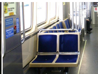
Priority seats and designated wheelchair securement areas, as well as emergency call buttons available within this area
