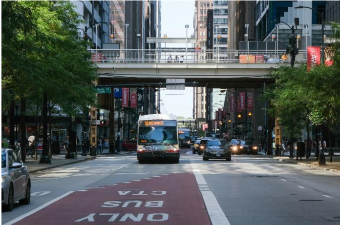
Identifying ways to prioritize CTA buses in heavily traveled corridors is a key focus of the Bus Priority Zones and Better Streets for Buses programs, which would leverage a variety of tools and street treatments, like bus only lanes.
