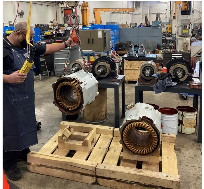
A CTA employee at the Skokie Heavy Rail Facility lowers a newly rebuilt traction motor onto a pallet. Work is part of the 5000-series quarterlife overhaul project.
